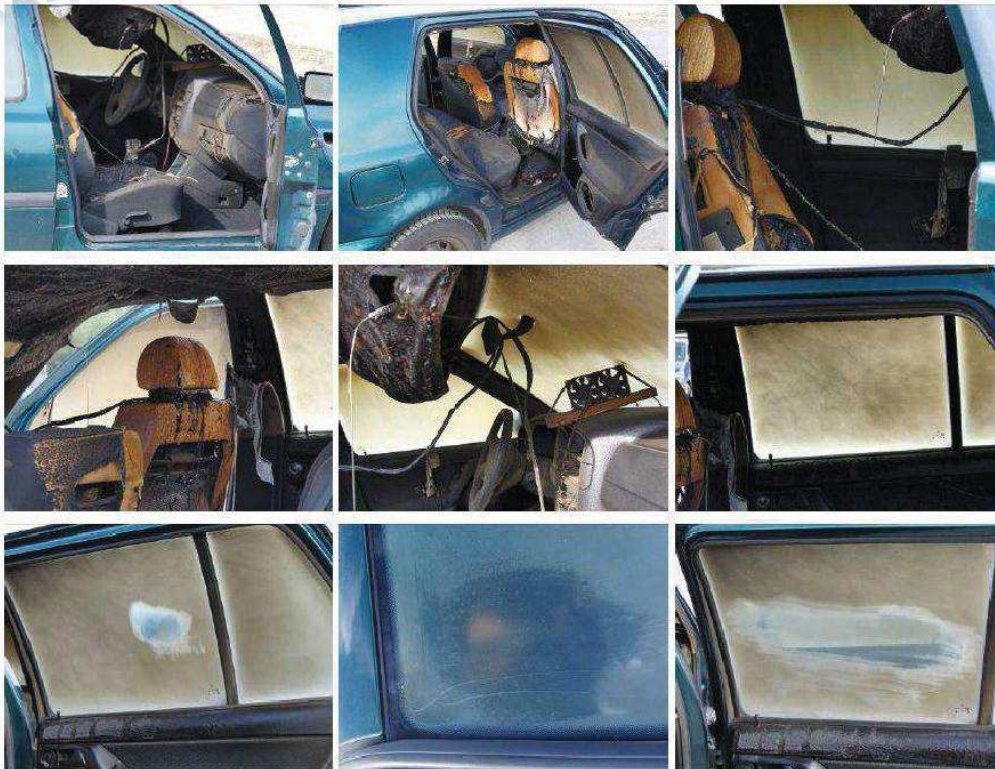
Fig. 29: Pictures taken after the combustion in the passenger compartment. Beside the typical view of such an event the translucent glasses caused by HF corrosion are impressive.
