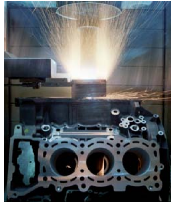
Nanoslide spray coating for engines
