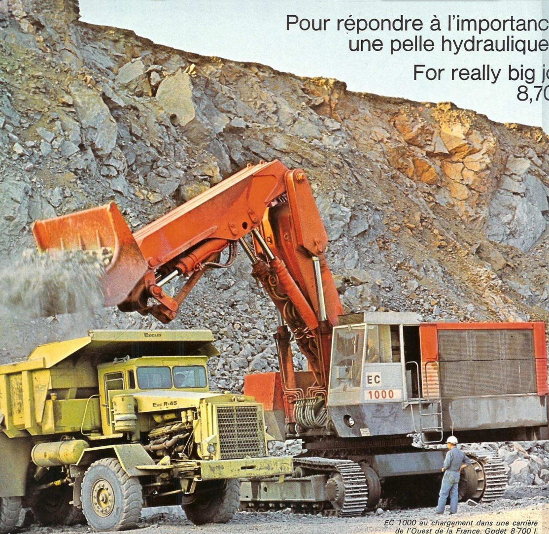
The Ec 1000 loading quarry material in the west of France on 8,700 l (11 1/2 cu. yd.) front loader equipment. Material : diorite (Deval. 27) - density in place 2.9 - 42 t. dumpers are loaded. Average hourly output : 1,000 t./hour.
