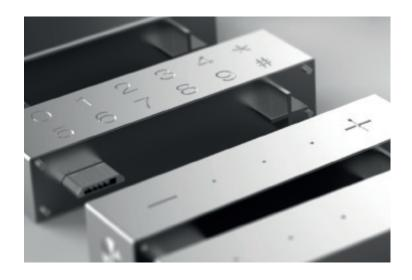
Unlike the current project as Ara, the concept of "-+" has no connection problem between elements. This is indeed a mini usb plug coupled to a structure "+" that provides the mechanical and electrical connection between each part of the handset. No more printed circuit previously managed all functions of the smartphone, at any time an element can be removed from the assembly without disturbing the rest.
