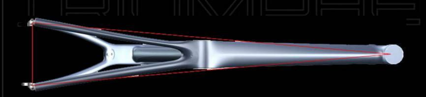
The Min/Max philosophy is also applied to the rear triangle. The chainstays are asymmetric because the drive and non-drive side stays are tasked with different functions when the bicycle is under pedaling load. Each is engineered to handle different forces and clearances. Chain force wants to twist the rear wheel in the dropouts.
