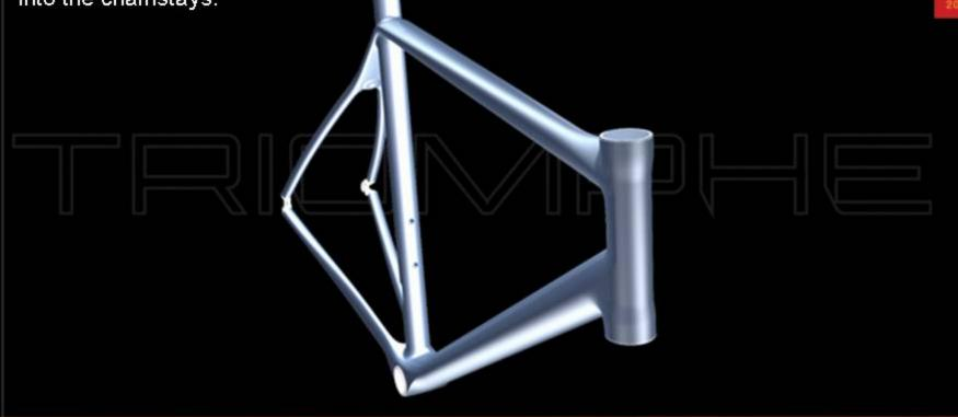
Both the top and down tubes, as they intersect the seat tube have maximum width in the horizontal plane, and minimum vertical height. The maximum width uses triangulation, the strongest geometric shape, to keep the head tube in the same plane as the seat tube. This results in precise and predictable handling. It also keeps the rear of the bike exceptionally stiff, transferring all the pedal input into forward motion.
