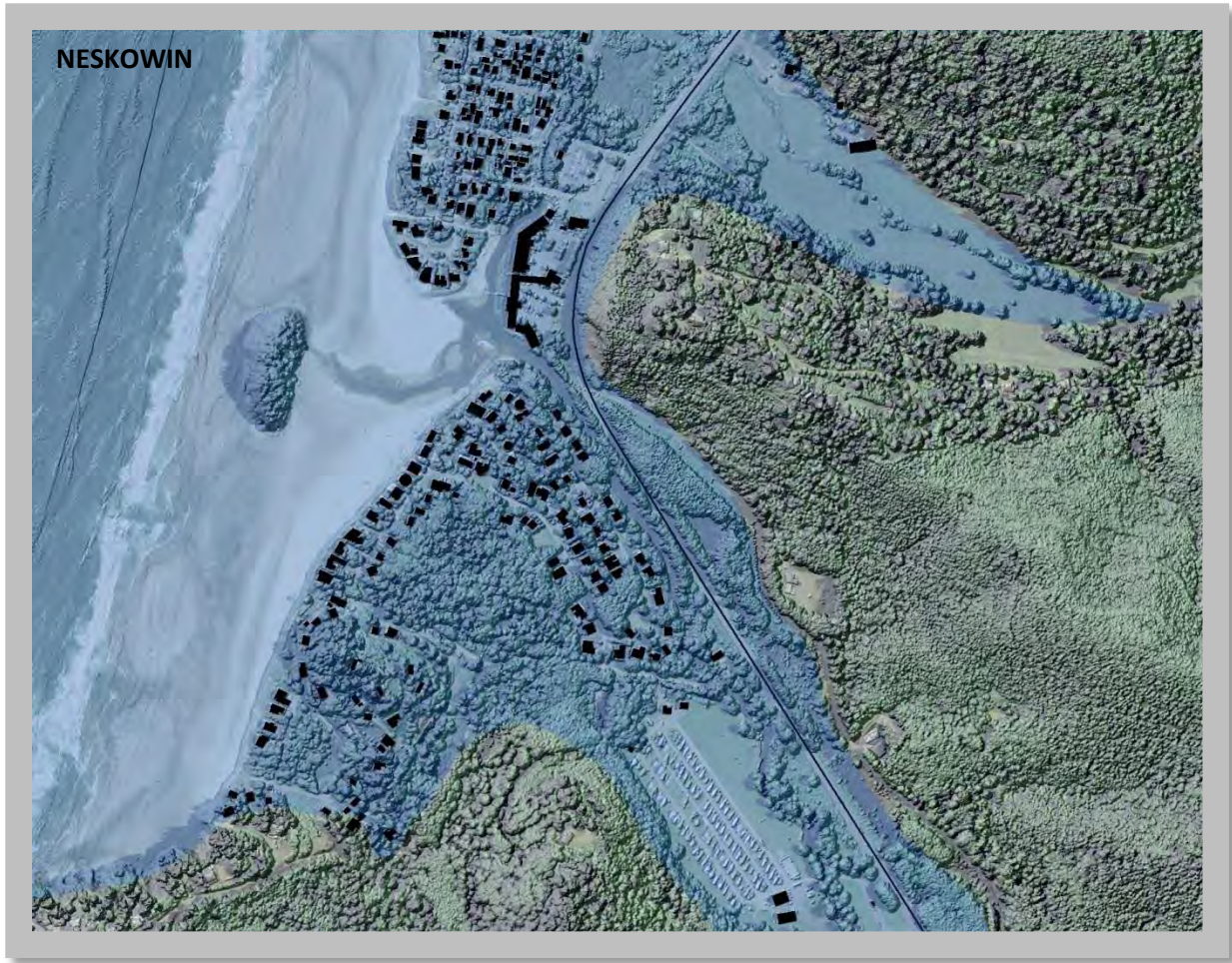
Figure 1.7: Estimated inundation of Neskowin due to the tsunami from the scenario magnitude 9.0 Cascadia earthquake. This tsunami map is based on the SB 379 regulatory inundation line.
